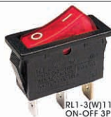
RL1-3(W)11/N-C-2-RE/BK-P2 ON-OFF 3P W/Lamp SPST
